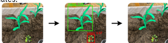
Figure 1: Example of the weed detection pipeline. Left: raw image. Center: neural network detections. Right: calculated laser target.
